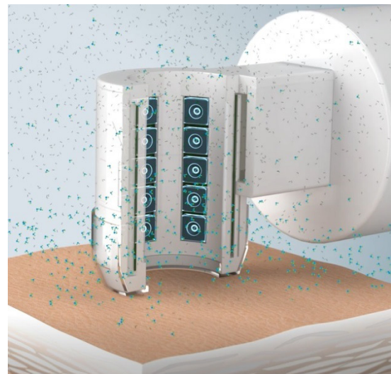
Fig. 1: Cross-section of an open-chamber probe (enlarged) (Tewameter; Foto: Courage & Khazaka, Cologne)
